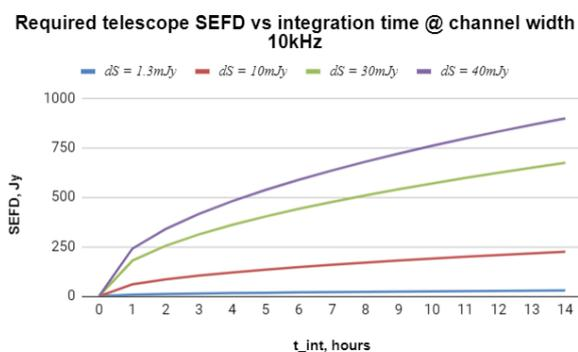
Fig. 2: Simulated Irbene RT-32 telescope sensitivity requirements for comet observation in single dish mode
