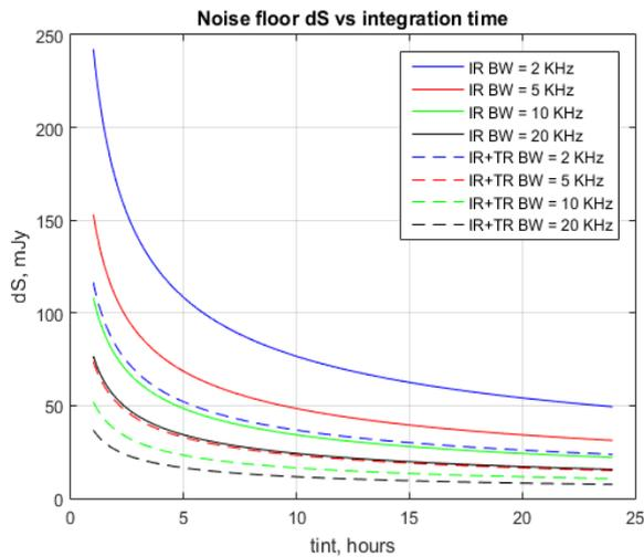
Fig.3. Achievable noise floor using Irbene RT-32 and Irbene-Torun interferometer vs. integration time and spectral resolution bandwidth
