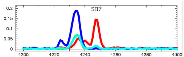
Fig.6. Cross-correlation functions for the baseline Irbene – Torun. Experiment date: 4 Feb 2019, frequency: 1660.49 MHz. Calibrator source 3C84 (left) and OH maser source W3(OH) (right). On the X axis - FFP points; on the Y axis - amplitude of the fringe function.
